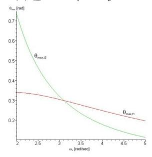
Figure 4  $\label{eq:figure 4} \mbox{Maximum $\theta$ angle values depicted as a function of the desired natural frequency value}$
