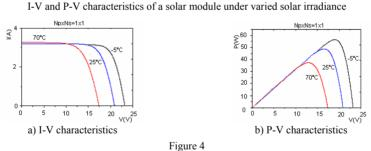
I-V and P-V characteristics of a solar module under varied temperatures
