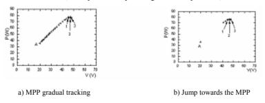
Figure 10 Experimental P-V characteristics, Es=56%, T=27 °C
