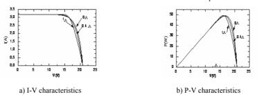
Figure 5 Influence of the series resistance Rs on the I-V and P-V characteristics of a PV module
