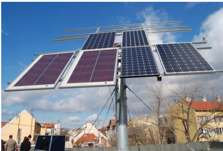
Figure 11. PV panel testing on Sun tracking system at Óbuda University
