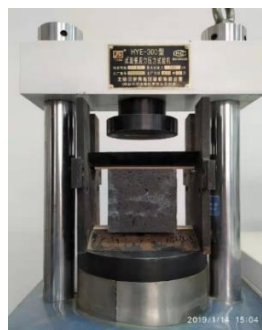
Figure 9 Splitting tensile test layout of concrete specimens
